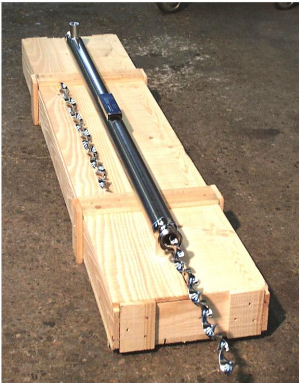
Fig. 3 CSE-W mixer/heat exchanger
