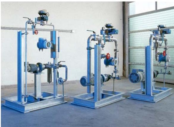
Fig. 3 KMD dosing modules in modular design for installation in a plant (installation and piping by the customer)
