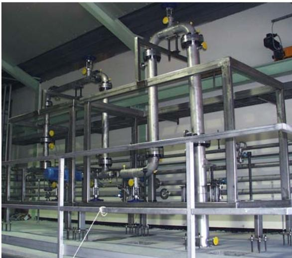
Fig. 4 Polymer plant with a KMD dosing module, static high-pressure mixers and a CSE-XR mixer/heat exchanger
