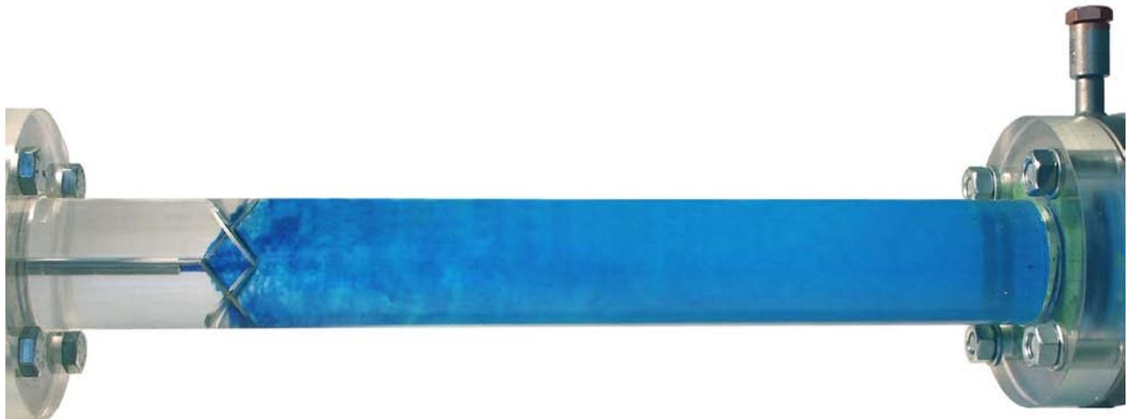
Fig. 1 5% blue additive is dosed upstream of a Milkmix mixer ( $Re = 18000$ )
