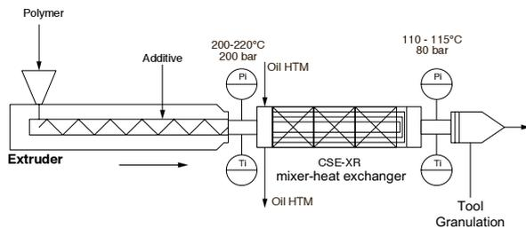
Fig. 5 Basic Scheme of the XPS-extrusion process
