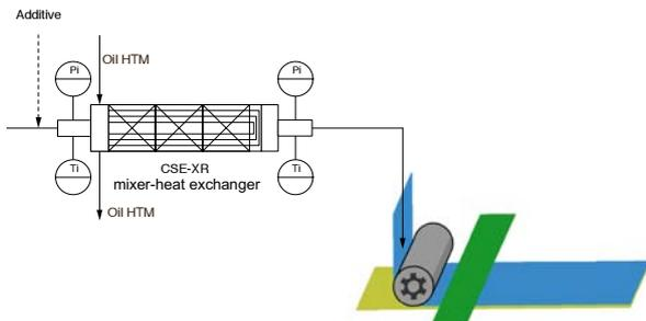
Fig. 3 Basic scheme of a coating plant
