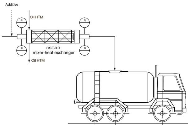
Fig. 4 Basic scheme of a filling plant
