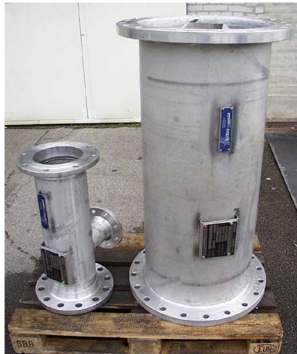
Fig. 4: CSE-B mixers with construction and pressure test
