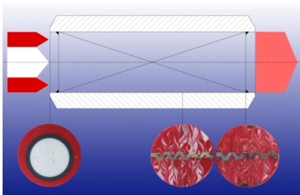
Fig. 1 Mixing performance of the CSE-X® Micro / Macro Fibre Mixer at a length of  $L/D = 2$  (2D-module) and at a length of  $L/D = 3$  (3D-module)
