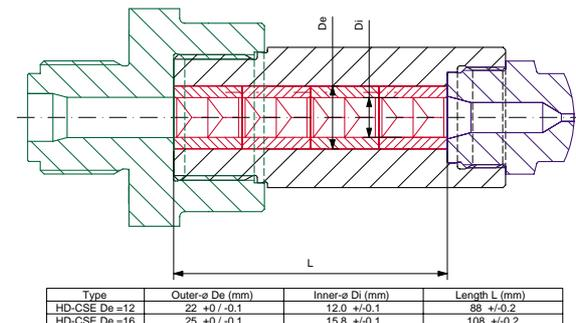
Fig. 4 Three parts HD-CSE mixing nozzle
