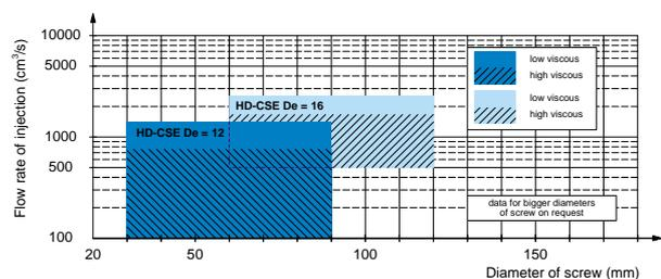
Fig. 5 Chart for the evaluation of the appropriate size of the mixing nozzle
