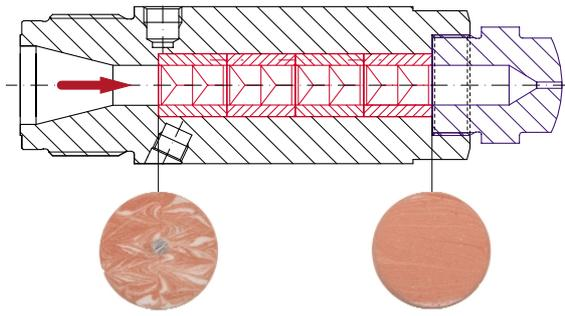
Fig. 3 Schematic illustration of the improved homogeneity of a two parts HD-CSE mixing nozzle. Epoxy cut to the left/right: inflow/outflow
