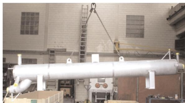
Fig. 5: CSE-XR® Polymer cooler
