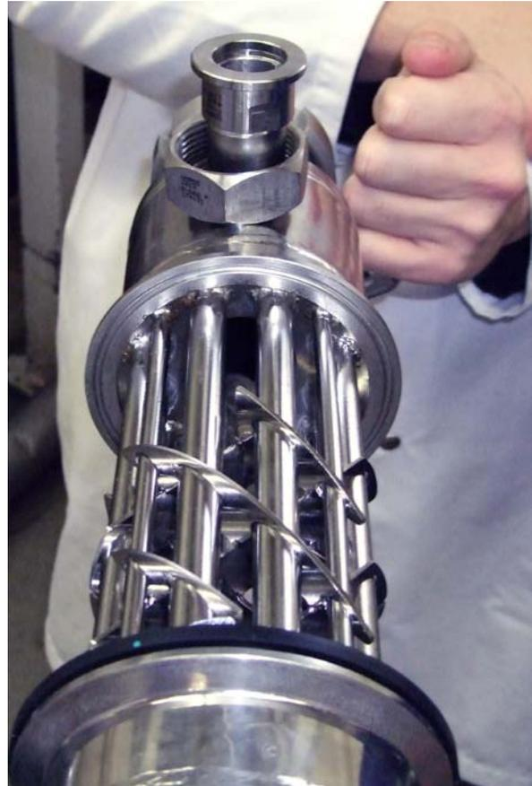
Fig 3: Inspection of the CSE-XR® by a client after CIP cleaning
