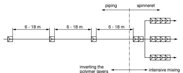
Fig. 2 First inverting, then mixing the polymer
