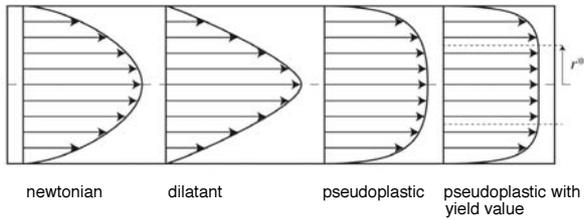
Fig. 3 Velocity profiles of polymers with different rheological properties
