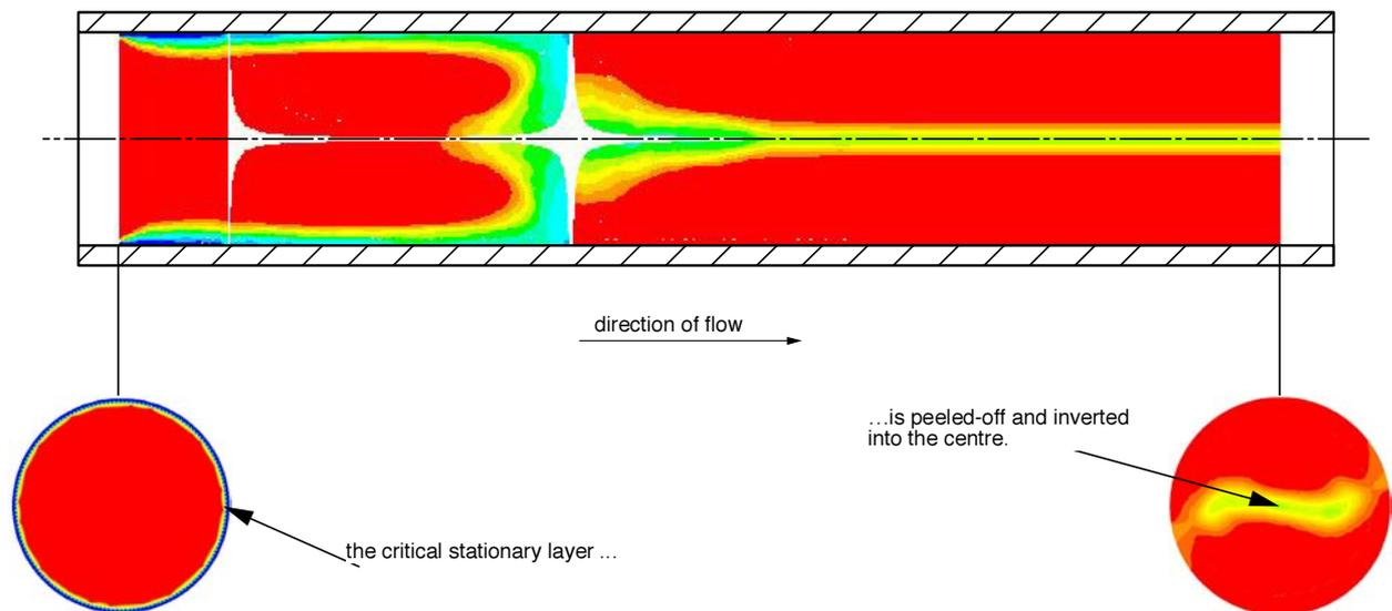
Fig. 1 CFD calculation of a Fluitec Polypeeler® for the inversion of stationary liquid films
