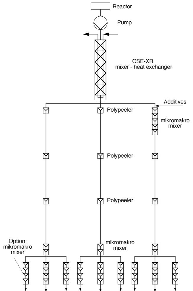
Fig. 5 Fibre-spinning plant acc. to Fluitec concept
