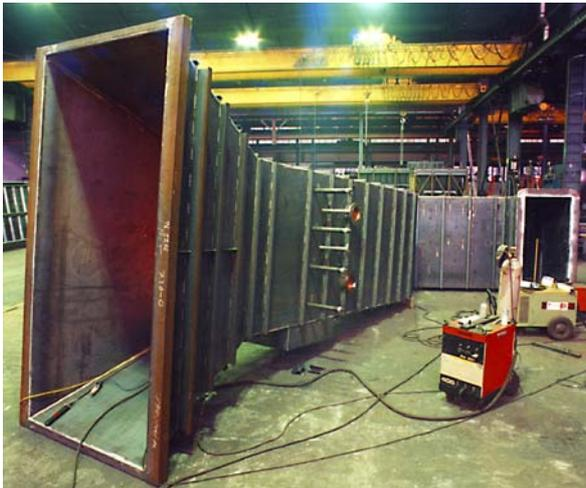
Fig. 4 Flue gas duct of a DeNOx plant
