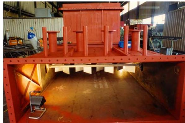
Fig. 6 Flue gas duct with static mixers
