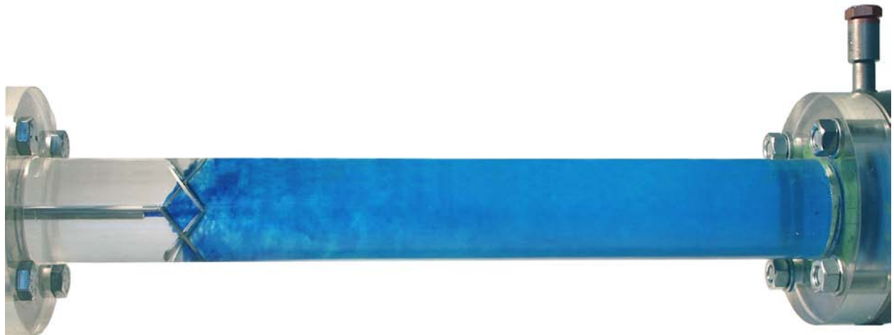
Fig. 1 5% of blue additive is dosed direct before an Aquamix/Flash Mixer ( Re = 18'000 )
