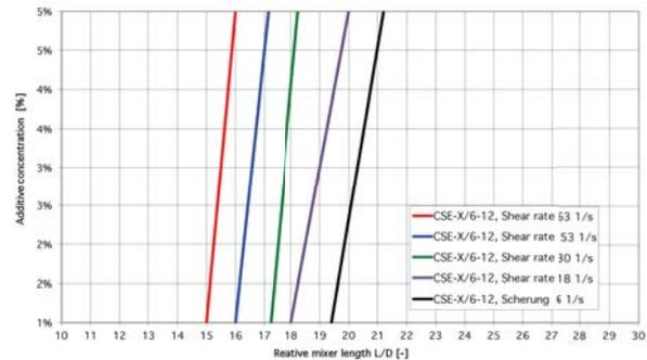
Fig. 7 Mixing efficiency of the new CSE-X mixer for a viscosity ratio of 35'000
