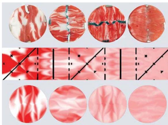
Fig. 1 Epoxy section and CFD calculation for the CSE-X/6-12 mixer
