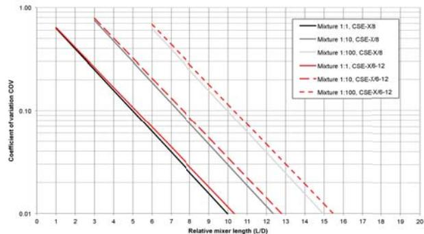
Fig. 4 Coefficient of variation COV of the Fluitec CSE-X and Fluitec CSE-X/6-12 mixers (adapted to the conductivity method [3], [2])
