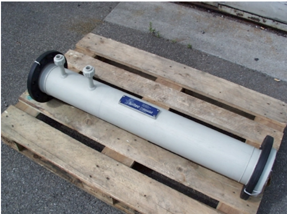
Fig. 2: Fluitec mixer with 2 dosage devices
