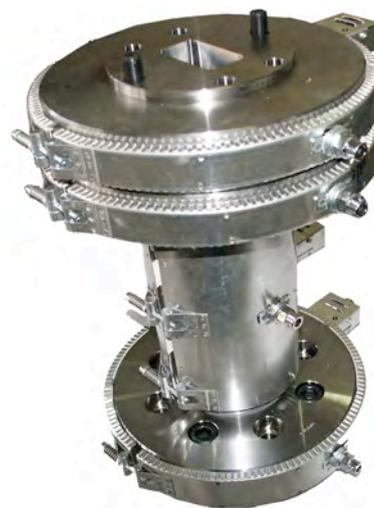
Fig. 5 Melt mixer with housing
