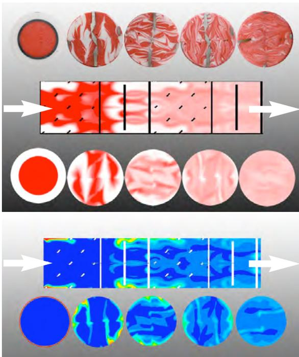
Fig. 4 Mixing performance of the Fluitec® melt mixer without wall effect.
