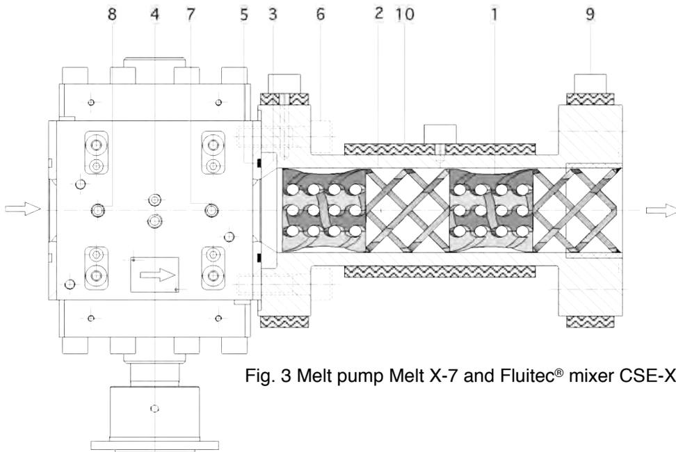
Fig. 3 Melt pump Melt X-7 and Fluitec® mixer CSE-X/4-09
