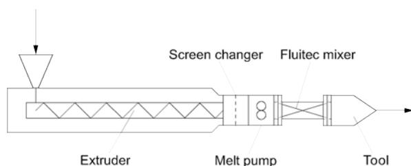
Fig. 1 Sketch of an extrusion plant
