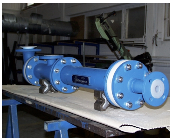
Fig. 6 FSB-Reactor, DN 100, PTFE lined
