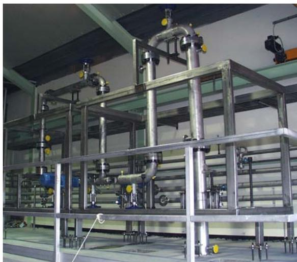
Figure 3 shows an isothermal loop reactor for a free-radical polymerisation. This Fluitec pilot plant has a capacity of 1500 tons a year.
