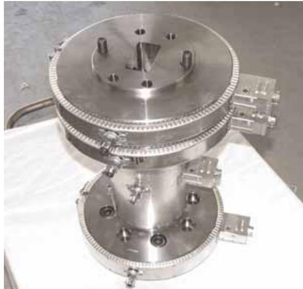
Fig. 6 CSE-X 90 melt blender with housing
